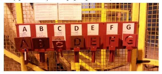
The visual mechanism comprised simple laser cut tags (*kaizen*) that travelled with subsets of heat treat families. At the end of normalising, the first free set of four tags (each of the same letter) would be put into the bin with the heat treat family, with the heat number and date written on the erasable back plate of the corresponding letter.
